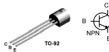
Figure 1: 2N3904 Pin configuration
