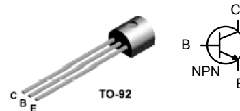
Figure 1: 2N3904 Pin configuration
