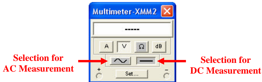
Figure 15: Multimeter properties window
